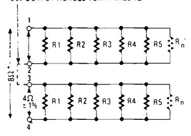
\*\*  $R_{TOTAL} = \frac{R}{n}$ , WHERE R IS THE RESISTANCE OF EACH RESISTOR AND n IS THE NUMBER OF RESISTORS
