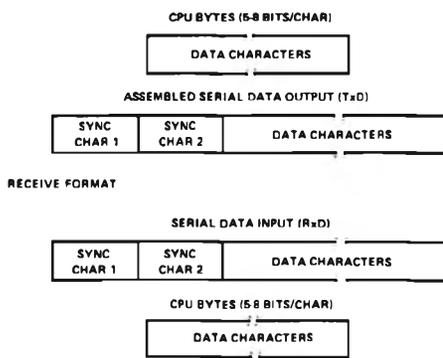
Figura 6 - 8251: synchronous mode, transmission format.
