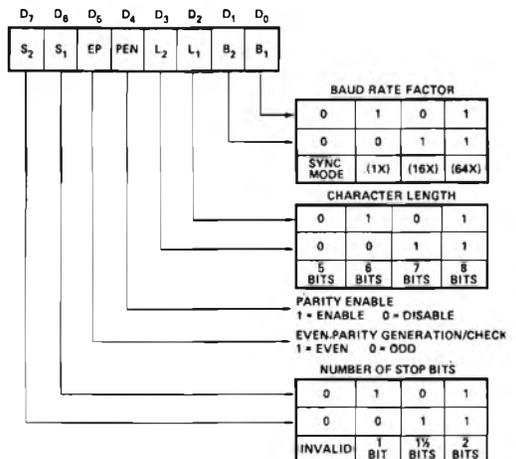
Figura 3 - 8251: mode instruction format, asynchronous mode.
