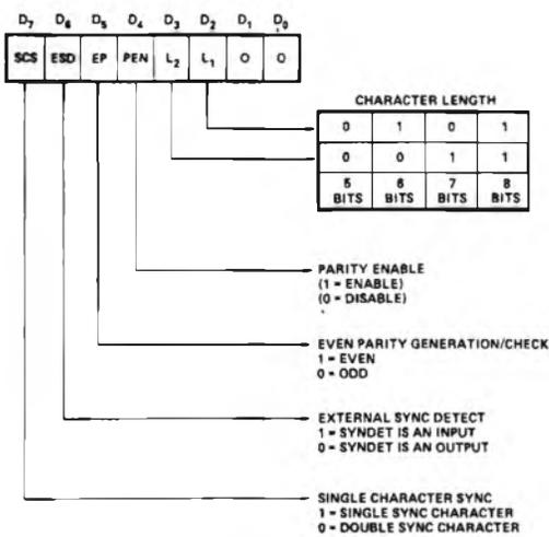
Figura 5 - 8251: mode instruction format, synchronous mode.
