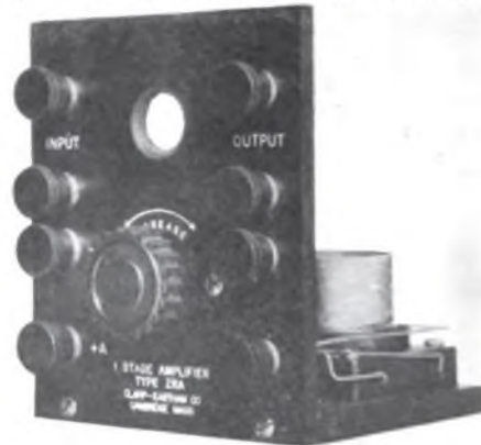
1-Stage Amplifier, bakelite panel, engraved in white, oak base.
