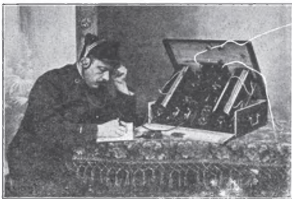
Here is Dr. Corret at a receiving station which he constructed in the French army during the war. In 1914 and 1915 he was in a little village in the Vosges. No tubes were available and he had to make use of cardboard tubes for the coils, odd bits of wire for the windings, wood rulers for the sliders, and he had even to make his square holes with a half-round file! In spite of which, however, this set worked very well and copied German messages which the headquarters set could not pick up.
