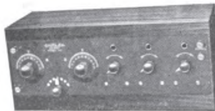
CROSLEY RECEIVER MODEL VIII-S. A new three tube set adapted to use 1½ volt dry battery tubes and eliminate storage battery. Consists of one stage of Tuned Radio Frequency Amplification, Detector and one stage of Audio Frequency Amplification in mahogany finished cabinet. Price without phones, batteries or tubes $50.00.
