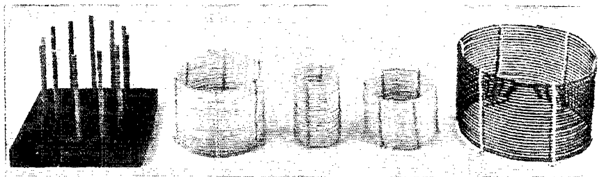
FIG. 1. THE WINDING FORM AND SOME OF THE COILS DESCRIBED IN THIS ARTICLE
