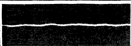
Oscillogram showing noiseless performance of BRADLEYUNIT resistors.
