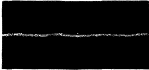
Oscillogram showing noiseless performance of Bradleyunit Resistors.
