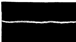
Oscillogram showing noiseless performance of Bradleyunit Resistors.
