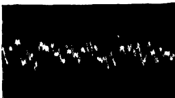
Oscillogram showing noisy performance of other types of resistors
