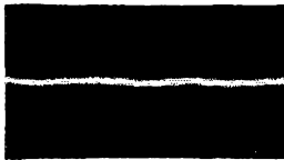
Oscillogram showing noiseless performance of Bradleyunit Resistors.
