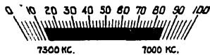
Showing here, the amateur, 1949 KC band is spread over the scale of the "278" receiver. The whole band covers only 20 KC in the ordinary, uncalibrated circuit, depending how permitted a spread of 16 divisions on the scale.
