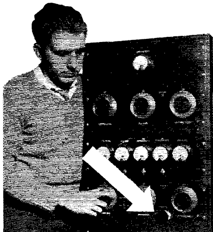
M. B. Kahn of the Collins Radio Company inspecting a Collins Transmitter furnished by the Byrd Antarctic Expedition. Arrow points to Bliley Mounted Crystal which is standard equipment on the set.
