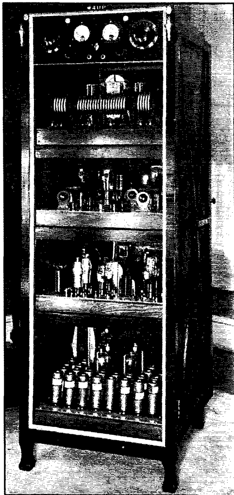
THIS COMPLETELY SELF-CONTAINED TRANSMITTER CAN BE OPERATED ON BOTH C.W. AND PHONE ON THREE BANDS
