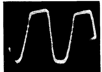
FIG. 5—A SINGLE-ENDED DRIVER STAGE GAVE THIS OSCILLOGRAM
