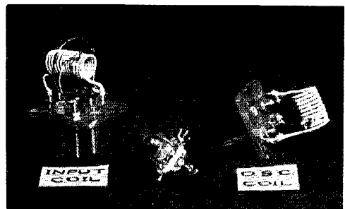
THE 28-MC. COILS USED IN THE ORIGINAL RECEIVER
