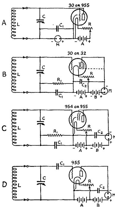
deflection to 50 microamperes from initial value. This holds the grid condenser discharge time within reasonable limits. The detector thus arranged is so sensitive that it may be necessary to keep one or two hundred feet from the transmitter and antenna when tuning to resonance with the fundamental frequency. A 30-microampere deflection occurred, for instance, 15 feet from the oscillator alone at WIES.
