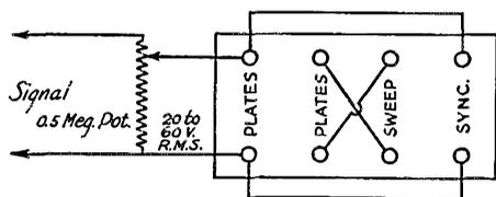
FIG. 4—CONNECTIONS FOR OBSERVING AN AUDIO-FREQUENCY SIGNAL VOLTAGE
