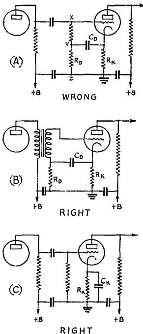
FIG. 1—THE WRONG AND RIGHT OF DECOUPLING CIRCUITS
