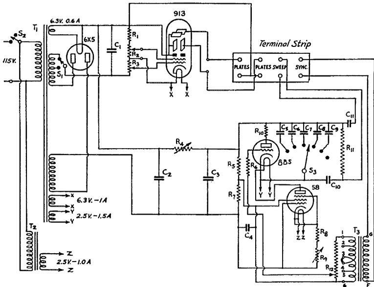
FIG. 1—COMPLETE CIRCUIT OF THE 913 OSCILLOSCOPE UNIT
