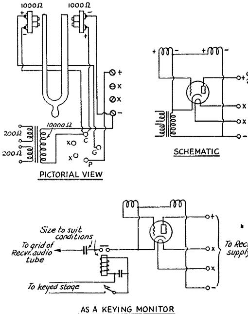
FIG. 1—CIRCUIT DETAILS OF THE TONE GENERATOR
