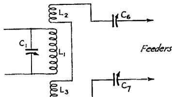
FIG. 2—ANTENNA COUPLING FOR ZEPP FEEDERS
