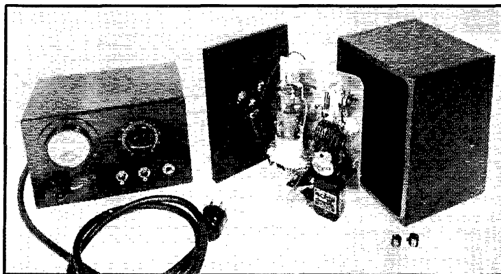
THE MODULATOR AND R.F. END ARE SEPARATE UNITS IN THIS 28-56-MC. PORTABLE-MOBILE TRANSMITTER
