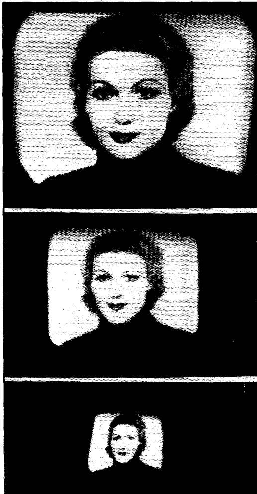
PHOTOGRAPHS OF THE IMAGE FROM A MONOSCOPE RECEIVED ON THE 906, 902 AND 913 CATHODE-RAY TUBES AND REPRODUCED AT APPROXIMATELY THE ORIGINAL SIZE
