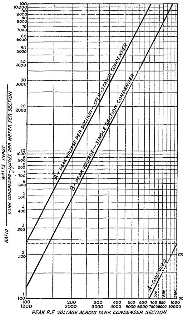
DETERMINING CONDENSER PEAK VOLTAGE
