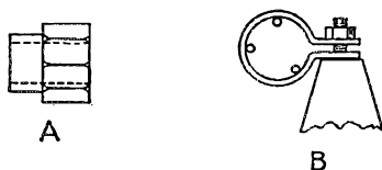
Fig. 1—Special threaded nut (A) and keyed clamp (B) for mechanism for remotely adjusting antenna-element lengths.
