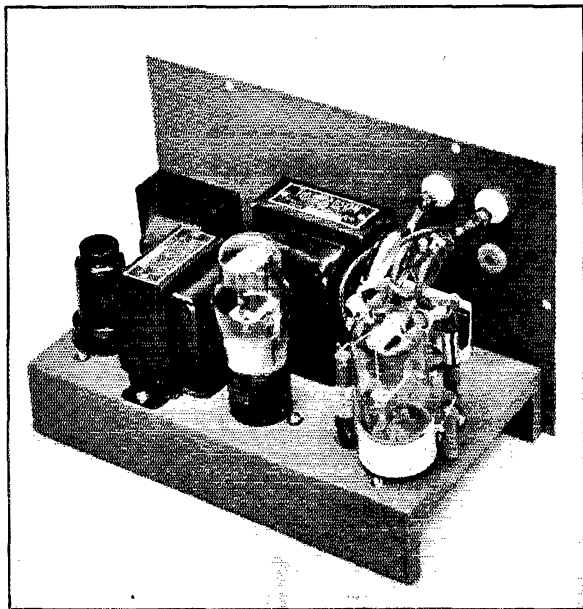
A rear view of the transmitter chassis.
