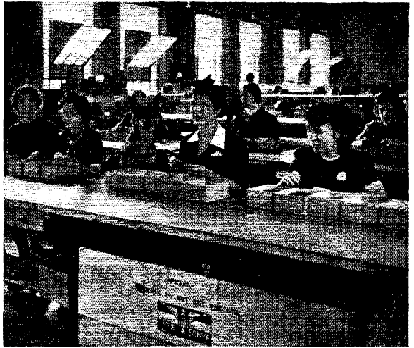
At Solar, blind women are more accurate than precision gages at inspecting mica spacers for flaws and grading them to tolerances of 0.0015 of an inch. Mary Murphy, second from right, veteran of the group, proved so efficient that other blind workers were added.
