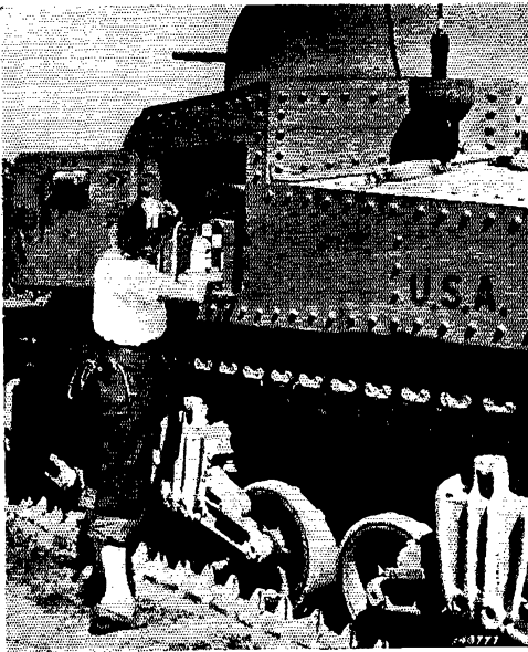
A Signal Corps lab technician services the f.m. transmitter in an M-3 tank. Official U. S. Signal Corps Photo.
