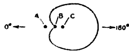
Fig. 1 — Field pattern from an end-fire system with 90-degree element spacing and 90-degree phase difference.
