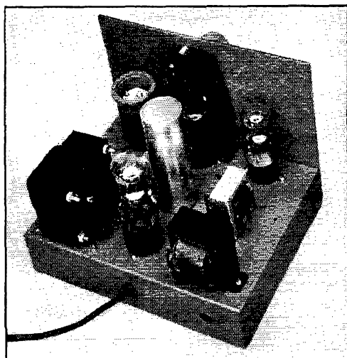
Rear view of the simple signal tracer. All power-supply components are mounted along the rear edge of the chassis. Close to the panel, from left to right, are the input coil and the detector and audio-amplifier tubes.
