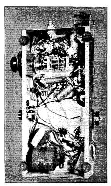
Bottom view of the WERS control-station receiver. The two acorn tubes in the h.f. circuits are visible above the tuning condenser, near the top end of the chassis. Power-supply components occupy the lower portion.
