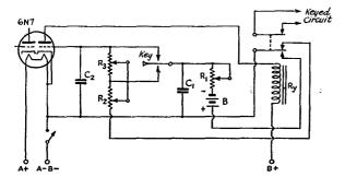
Fig. 1 — Circuit diagram of the simple electronic key.  $C_1 - 2 \mu f d$ . B - 3-volt battery.  $C_2 - 0.01 \mu f d$ . Ry - Sensitive-type relay.  $R_1$ ,  $R_2$ ,  $R_3 - 100,000$ -ohm potentiometer.
