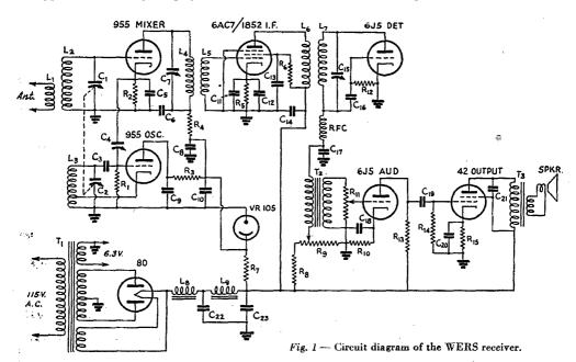
variable (see text). C<sub>8</sub>, C<sub>6</sub>, C<sub>16</sub>—100-µµfd. midget mica. C<sub>4</sub>, C<sub>7</sub>, C<sub>18</sub>—3-30-µµfd. trimmer. C<sub>8</sub>—50-µµfd. midget mica. Cs, C10, C17 — 0.001-µfd. midget mica. Co - 500-μμfd, midget mica. Cit - 0.002-µfd. midget mica. C12, C13, C14 - 0.01-µfd. 400-volt paper. <sub>0</sub> — 25-µfd. 25-volt electro-C1 & C20 lytic.
