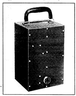
The 112-Me. m.o.p.a. transmitter for WERS is entirely enclosed within its standard metal carrying case. The male-plug receptacle near the bottom is for power-supply connections. Tuning adjustments are made by screwdriver through holes in the regr of the case.
