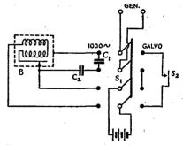
Fig. 4 — Circuit of the 1000-cycle tone source.
