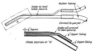
Fig 3 — Constructional details of the homemade soldering torch.
