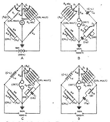
Fig. 2 — Basic bridge circuits. Λ — Wheatstone bridge used for resistance measurements. B — Capacity bridge for measuring capacity and power factor. C — Maxwell inductance bridge. D — Hay inductance bridge.
