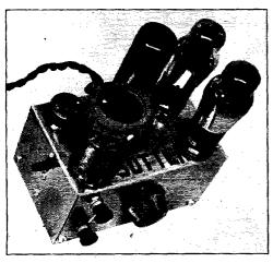
Top view of the 15-watt midget rig. The two tubes at the right are the rectifier tubes for the voltage-quadrupling transformerless supply. The 616 oscillator tube is behind the coil in the foreground and the crystal occupies the rear left-hand corner of the chassis. The plate-tank tuning knob and key terminals are mounted on the front. On the left edge is the band-change switch.
