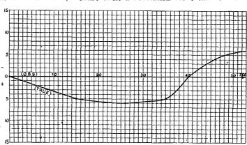
from the readings. This may be done either by using the true positions of the stakes as a reference axis and plotting the deviation of the bearings against it, or by using the observed readings as the reference axis and plotting the true bearings against that axis. Either method is satisfactory. The second method was used in plotting the sample curve shown in Fig. 1.
