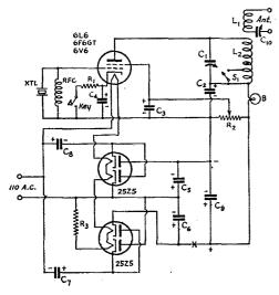
Fig. 1 -- Circuit diagram of the midget transmitter. C1 - 100-μμfd. midget variable (Hammarlund Star). C<sub>2</sub>, C<sub>3</sub>, C<sub>4</sub> — 0.01-μfd. 600-volt tubular paper.
