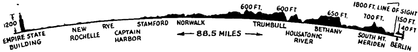
Fig. 1—Cross section showing the signal path between the Empire State Transmitter and the author's home in Berlin, Conn. The receiving antenna is approximately 1000 feet below the line of sight.
