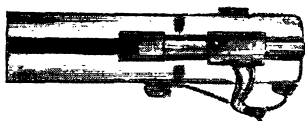
Interior View showing crystal element, Nylon chuck and sapphire-tipped, knee- action Nylon needle and metal needle guard.
