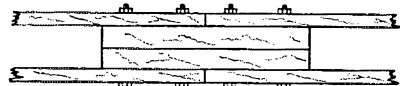
Fig. 2 — Sketch showing the method of splicing the two sections of the mast.
