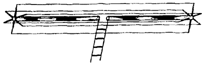
Fig. 1 — Sketch showing the essential plan of constructing a multi-element cage antenna for use as the radiator in a close-spaced array.
