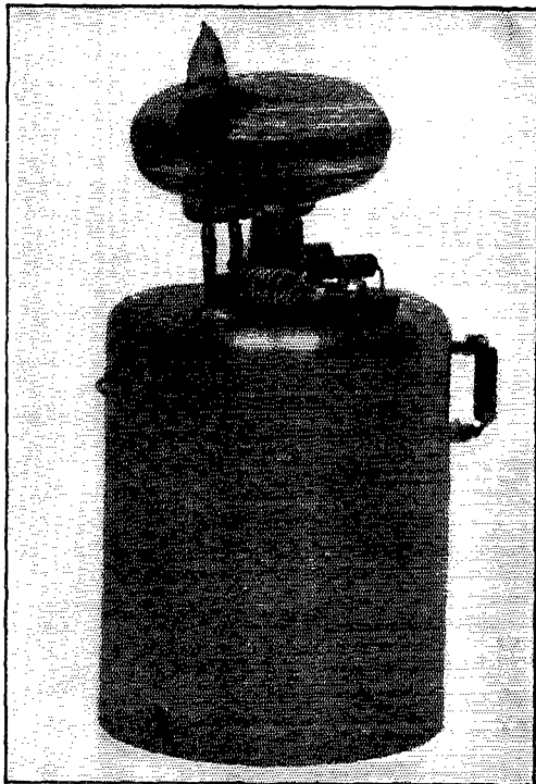
The oscillator assembly with the 703A in place. The grid leak, R_2 , is at the right.
