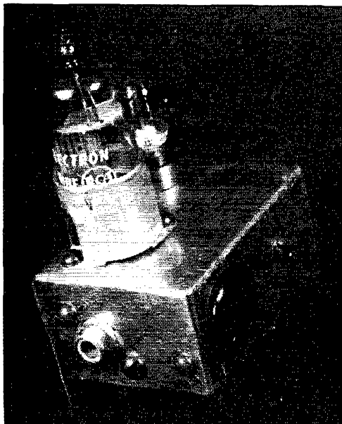
The simple keying monitor can be built so small that it will fit into any receiver. The Jones fitting below the 6AQ6 tube takes the r.f. pick-up line.
