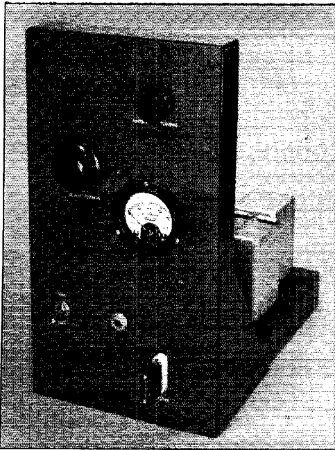
Fig. 5 — Front view of the rack-and-panel version of the transmitter. Strips of 1 \times 2 are used for the uprights and side rails of the frame, while the side brackets are made of \frac{1}{4} -inch Presdwood. Thin strips nailed across the side rails support all of the power-supply components, and all of the transmitter parts are bolted to the front panel. The framework is 13 inches high, 11 inches deep, and 7 inches wide.
