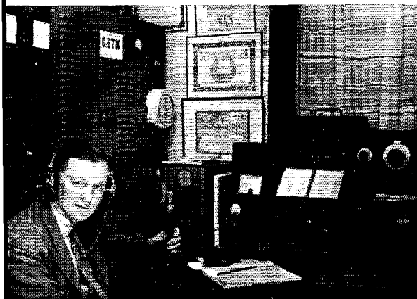
Belfast's G16TK, operated by Frank Robb, has long been a standout on any band when Europe is coming through. Equipment shown here is capable of operation on all bands, 3.5 through 60 Mc. An 808 final is generally used; receivers include an HRO, AR88 and CR100.
