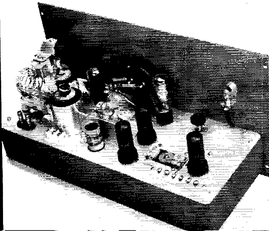
The 28-Mc. bandpass filter is in place in this rear view of the transmitter.
