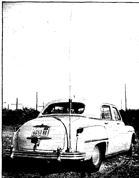
A high-efficiency antenna for 75-meter mobile work. The center-loading coil is tuned precisely with a built-in adjustable condenser.
