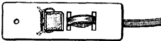
Fig. 1—A sturdy end-insulator for folded dipoles made of Twin-Lead. In addition to providing secure anchorage for the end of the dipole, a convenient mounting place for a fixed mica condenser is available.
