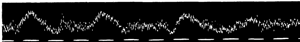
Aurora-propagated 50-Mc. signal of W1HDO, as recorded at Ithaca, showing rapid fading. The evenly-spaced markers (bottom) are 120 per second. At about 2300 on Feb. 26, 1951, when this record was made, voice was completely unintelligible. Earlier in the same evening voice had been partially readable, the signal curve being much smoother at that time.
