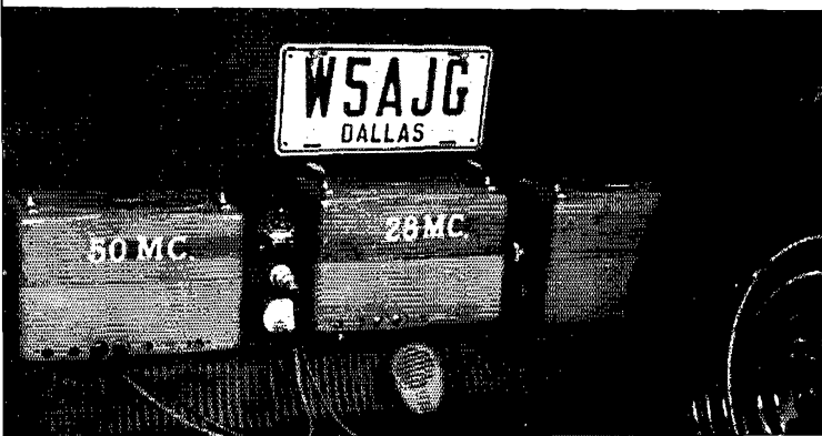
The two-band mobile installation of W5AJG, Dallas, Texas, using two police transmitters converted for operation on 28 and 50 Mc. A microphone and metering position are provided for tune-up purposes.
