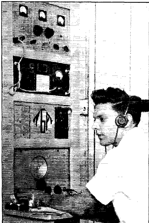
Like Scrutan, VP6PV's call makes sense backwards. Paul likes c.w. but can screen-modulate his 807 final and has been widely worked on most DX bands. (Photo by W24IS)
