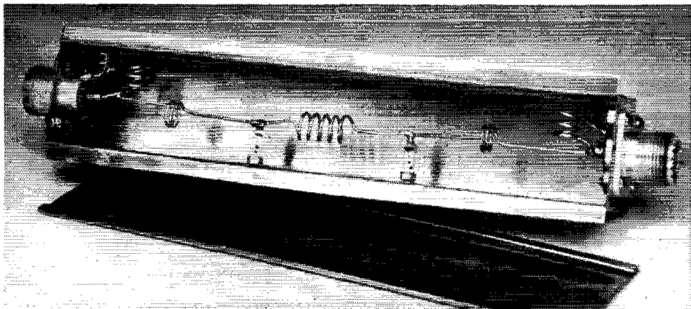
Low-pass filter for use with low-powered 144-Mc. transmitters. Maximum attenuation is in the region of 190 to 215 Mc., but good from 170 Mc. up.
