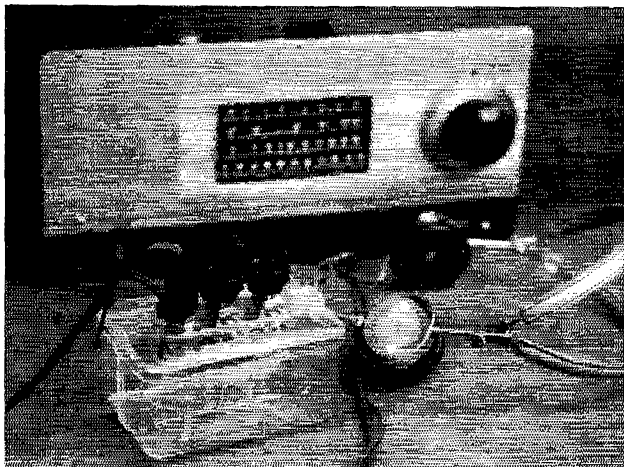
View of the filter ready for use. The plastic box makes a neat chassis and also serves to keep dust off the parts.
