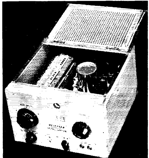
Top view of the Signal Shifter, showing the home-made shield can over the 807. Also shown is the strip of metal forming the lip at the rear of the opening to seal the slit along the hinge.
