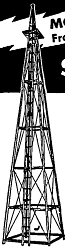
Width of Base Equal to 1/5 Height
