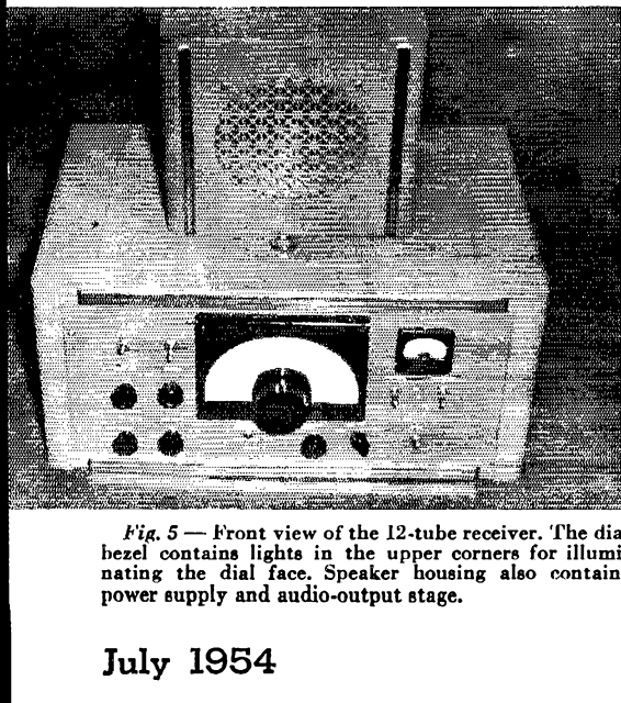
Fig. 5 — Front view of the 12-tube receiver. The dial bezel contains lights in the upper corners for illuminating the dial face. Speaker housing also contains power supply and audio-output stage.
