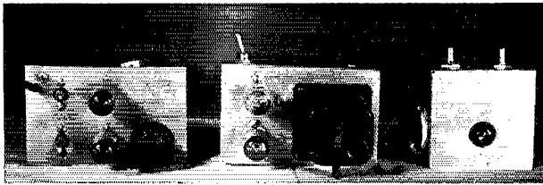
Subassembly construction made mass production of the 2-meter rigs possible for KBT club members. The combined audio-modulator unit, center, is flanked by the transmitter r.f. section, and the receiver front end.
