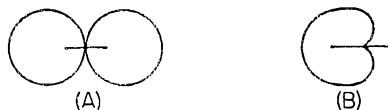
Fig. 3 — Loop field pattern. A — Without sense antenna. B — With sense antenna. The horizontal lines show the plane of the loop.
