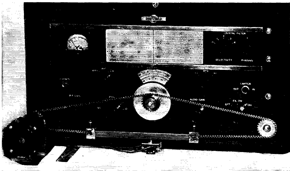
The automatic band-scanner installed on a Collins receiver. The motor-driven chain that operates the tuning shaft of the receiver carries adjustable stops that actuate a reversing switch. As much or as little of the band can be monitored as desired.
