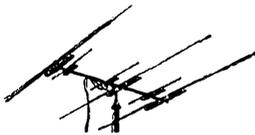
**10 and 20 METER BEAM** — Provides top performance on two favorite DX bands. 3 elements for 10 and 20 are interlace mounted on one boom. Feed both beams with just one 52-ohm coax line — switch bands at transmitter. Pre-tuned to 3 frequency ranges in each band. 7 1/2 db forward gain, 28 db front-to-back. 1.5/1 SWR or better at resonant freq. Max. element length 22 1/2". Less mast, rotor and coax line.
