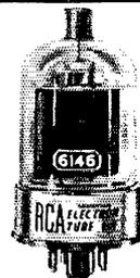
RCA-6146 Amateur radio's most popular power tube. 90 watts input, CW; 67.5 watts, 'phone.
