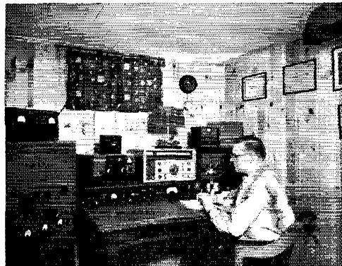
NNJ Official Bulletin Station W2VCZ rolled up the January CD Party's leading phone score at this well-appointed operating position. Gear includes a kw. final and modulator, Ranger, NC300, Viking I and v.f.o. These are intermittently tied to 10-11 and 15-meter rotaries, and to fixed arrays on 40 and 80.
