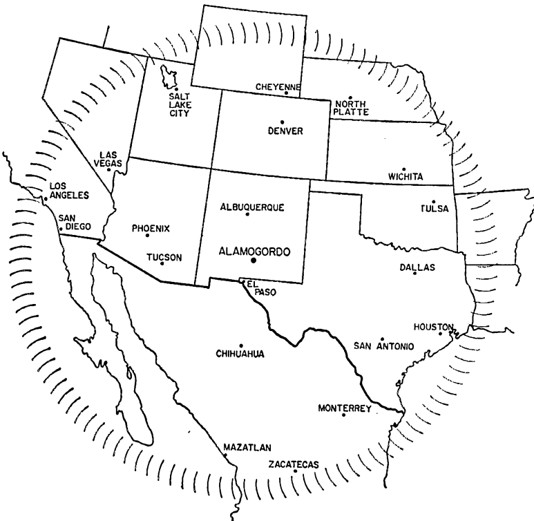
Fig. 1 — Communication by reflection from the artificial ion cloud should be possible within the area bounded by the diffused-outline circle.
