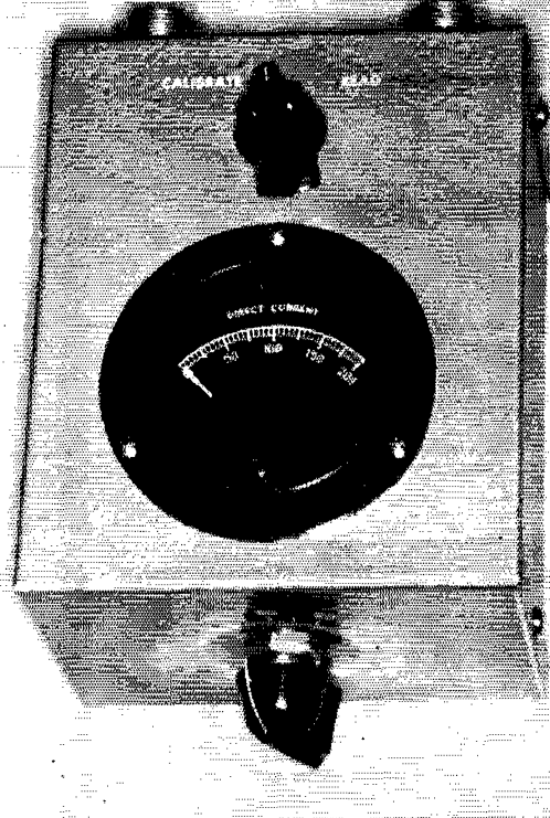
This s.w.r. indicator features simple construction using ordinary coax cable. The forward-reflected switch—labeled "Calibrate" and "Read"—is at the top. The control below the meter is the sensitivity control.
